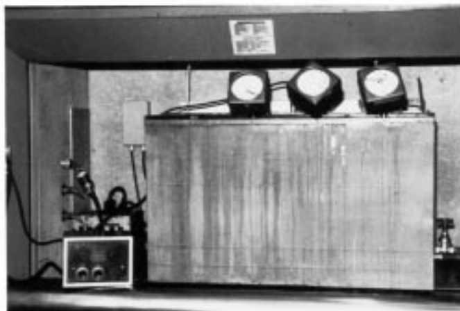
FIG. 1 Rotating Bomb Oxidation Test Apparatus
