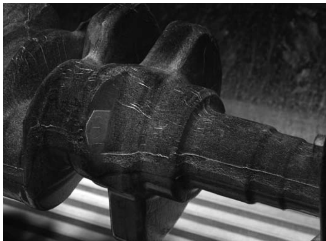
FIG. A1.4 Crankshaft with Various Longitudinal Indications
